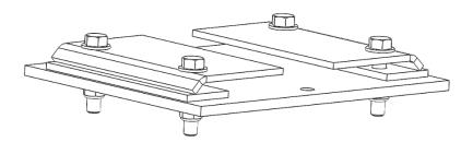
5. Install bottom plate [EN823X8328] with I-beam clamps assembled through center holes onto the two threaded rods using  $\frac{1}{2}$ " nylock nuts and a flat washer allowing enough space for the web truss beam to easily slide through the assembly.
