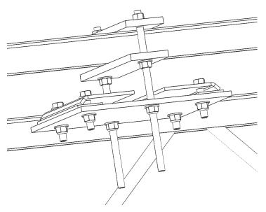
6. A minimum of two mounting points are required to carry the various lengths of web truss beam assemblies. Repeat steps 1-5 as required.
