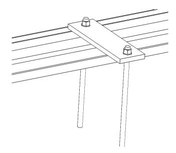
3. Install 3" flat bar without nuts through the holes onto threaded rod using ½" nuts and flat washers, thus sandwiching the top chord of the truss. Torque nuts 12 ft/lbs [as per details].
