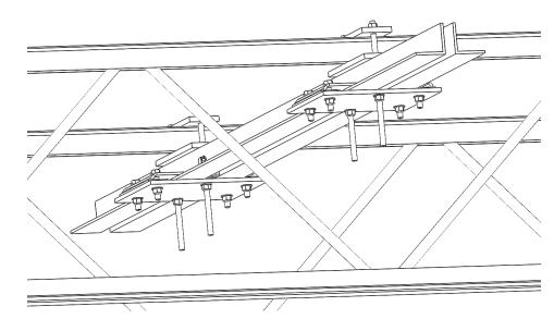
9. Thread safety cable around beam assembly and top chord of truss at each mounting point. Fasten the safety cable by looping the cable ends together as shown in detail and clamping them together using 3/16" cable clamps.
