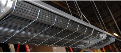
Two sections make up the protective guard assembly that installs on the underside of the P40-U heater. Near the bottom edge at each side of the reflector are two sets of three holes. Each set of holes has one round hole at the center of the reflector, the other two holes are elongated and positioned between the center and the ends of the reflector. The pins that extend from each side of the two guard sections are inserted into these sets of holes.
