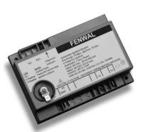
When flame is detected during the trial for ignition, spark is shutoff immediately and the gas valve remains energized. The thermostat and main burner flame are constantly monitored to assure the system continues to operate properly. When the thermostat is satisfied and the demand for heat ends, the gas valve is de-energized.
