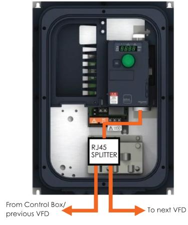
\* Connect Cat5 Cable and splitter to port inside of VFD enclosure
