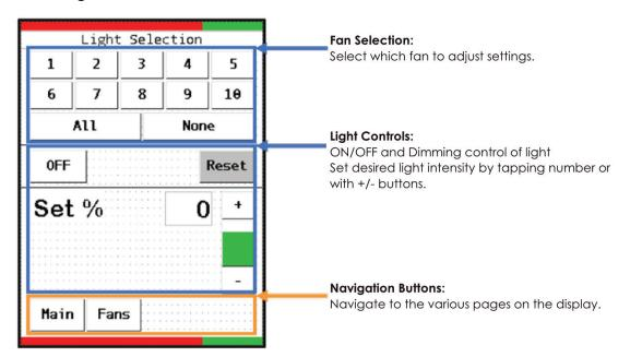
Note: This screen is only accessible if the unit is equipped with the LED light option.
