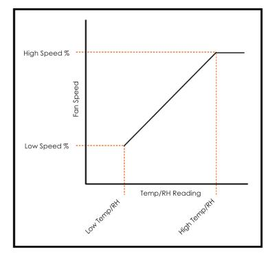
This chart shows how the fan speed is calculated relative to the sensed temperature and humidity
